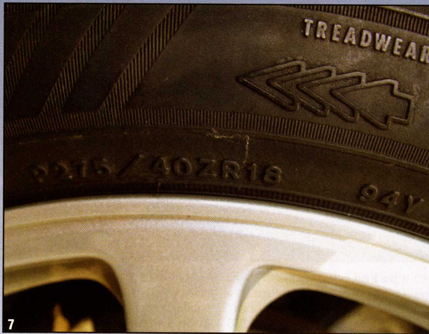
This illustrates a speed rating of "Y" for a P275/40ZR18 rear tire from a 2000 Corvette.
