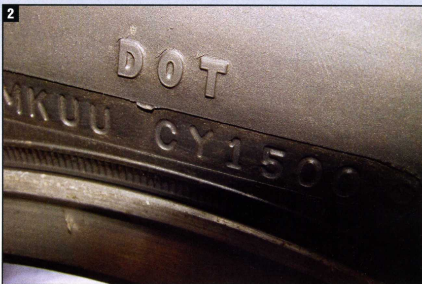
2 A typical 1980 P255/60R15 date code shows that tire assembly still used a single gang (actually called stencil plate) to mold the TIN into the tire. The DOT label is printed on the topside of the TIN. This tire was manufactured the 50th week of 1980.
